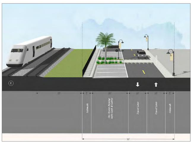
In the concept above the existing sidewalk to the west and the FEC Railway including the 25' clear zone remain the same. Within the Town's right of way a new fence, sidewalk, curb and gutter are added to improve safety along the FEC Railway. The concept also illustrates an opportunity to add pervious pavers to the on-street parking with an enhanced mid-block crossing.
